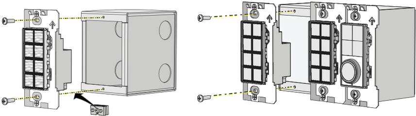
1. Insert the station electronics and wiring into the back box. To install multiple stations (multi-gang), insert the station electronics into the back box from the right to the left side for the best alignment and fit. The alignment bracket will slightly overlap the station to the right when properly installed.
