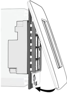
1. Align the top of the wall plate to the station and angle the bottom approximately 20 degrees.
