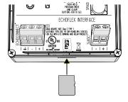
3. Cycle power to the unit. The INPUT STATUS, LEARN/TEACH, and PROGRAM MODE LEDs flash to indicate the update process has begun. After several seconds, the OUTPUT STATUS LEDs illuminate to indicate the progress of the update.
