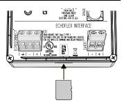
3. Cycle power to the unit. The INPUT STATUS, LEARN/TEACH, and PROGRAM MODE LEDs flash to indicate the update process has begun. After several seconds, the OUTPUT STATUS LEDs illuminate to indicate the progress of the update.
